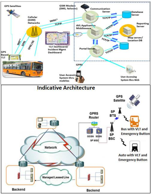
A suitable control mechanism would be established for the data transfer from VLT to Backend Control Centre, as only the authorized devices should be able to transfer data to the Backend Control Centre and a mechanism for authenticating the devices/SIMs shall also be put into place.
